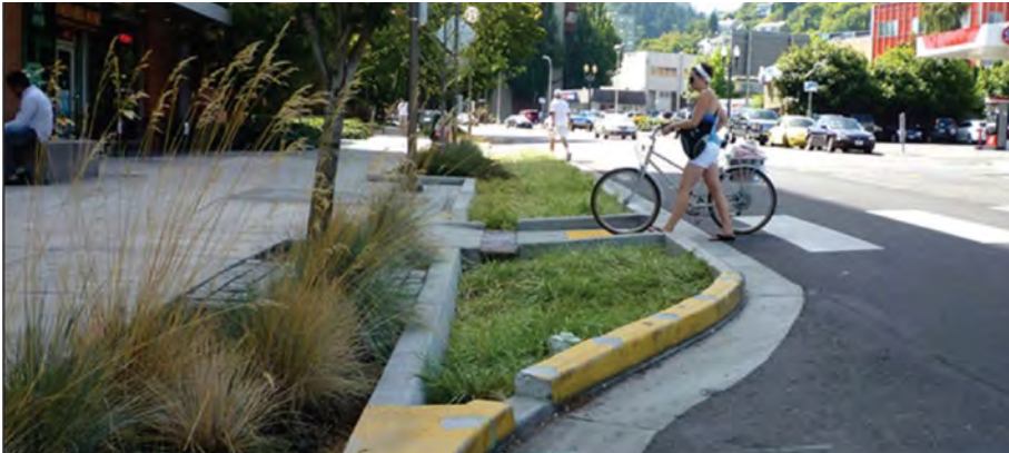
Figure 5. Stormwater Curb Extension (Source: NACTO)
